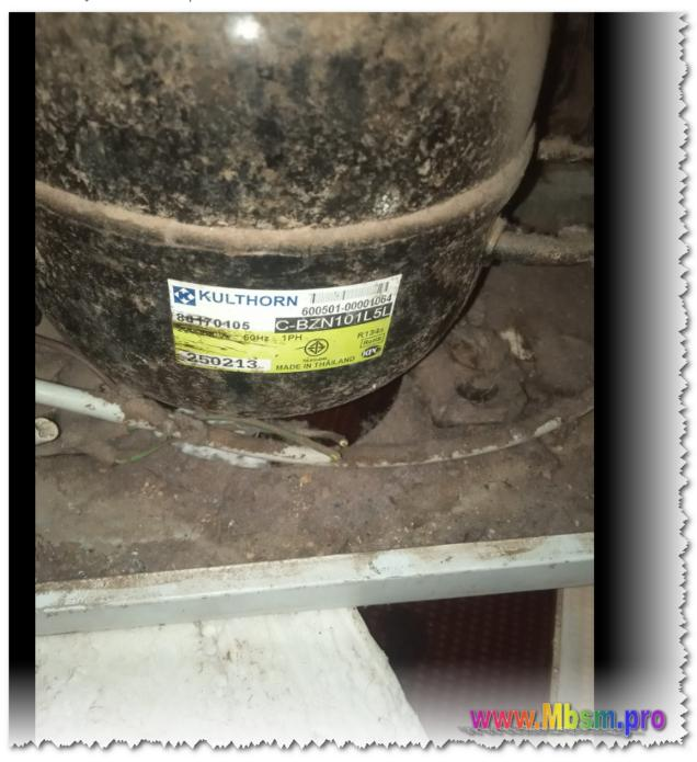
c-bzN101 appears to be a model number for a KULTHORN refrigerator compressor. It's specifically a 1/8HP compressor, which is commonly used in smaller
