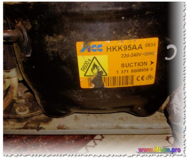
The **Comp HKK95AA** is a compressor designed for refrigeration applications, specifically operating at **220-240V** and **50Hz**, with a capacity of **1/5 HP** (**167W**) and using **R600a refrigerant**. Here are some key details:
