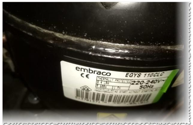
The **EGYS110CLC** compressor has a power rating of **1/3 HP** (horsepower) and is designed for low-temperature applications. Here are some key specifications related to its horsepower and performance:
