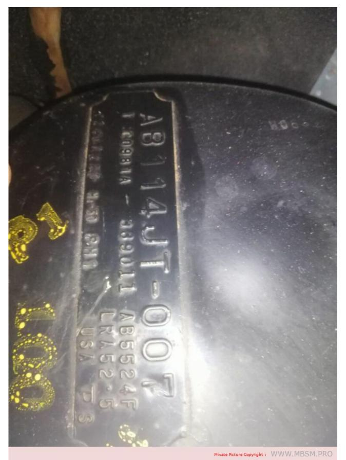
The AB114JT compressor is a Tecumseh 2 HP, 208-230V, 1 PH, 24200 BTU, R22, Hermetic (Reciprocating) Compressor Replacement. It is available for purchase from AC Parts Distributors[1][2]. It is also listed in a compressor substitution guide[5]. However, it is not clear what the specific application of the compressor is or what equipment it is compatible with.
