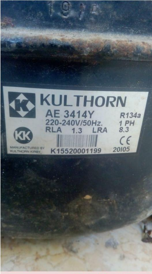
Private Picture Copyright: WWW.MBSM.PRO Mbsm.pro, Kulthorn, AE 3414Y, Compressor, Small, 1,570 BTU/Hr, 1/8HP, R134a, 208-230V, 60Hz, 1Ph, HBP, overload Plus Relay, AE3414Y **Description**
