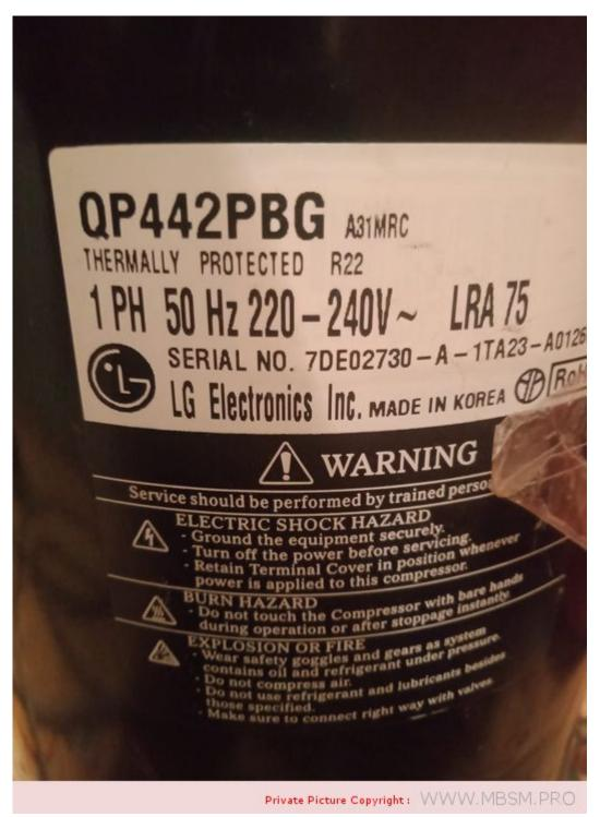
Mbsm.pro, Compressor Lg, 26000 btu/h, QP442PBA, LG, AC Rotary Compressor, Rotary Scroll Compressor, 220-240V 50HZ, 2 ton, 3 Hp, 1 PH
