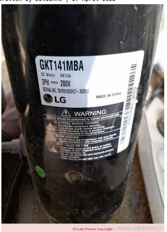
Mbsm.pro, GKT141MBA, Compressor , LG, inverter, BDC, DC compressor, 3 PH, 2.5 HP, 18000 Btu/h, R410A
