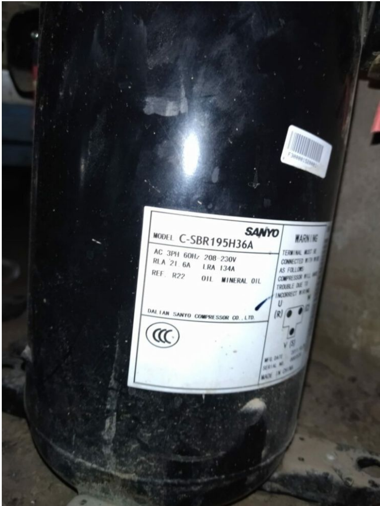
Mbsm.pro, compressor, Scroll Sanyo, C-SB, C-SBR195H38A, 5.5 hp, 400 v, 3 ph
