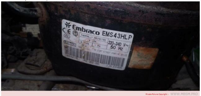
Mbsm.pro, Compressor, Embraco, Aspera, EMT43HLP, EMY3111Z, LBP-R134a, R507, 220-240V/1/50Hz, 1/8and HP, displacement 4.85 cm3, motor type RSIR
