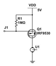
Motor connected from transistor to -V/GND
