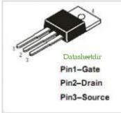
Type Designator: IRF830 Type of Transistor: MOSFET Type of Control Channel: N -Channel Maximum Power Dissipation (Pd): 100 W Maximum Drain-Source Voltage |Vds|: 500 V Maximum Gate-Source Voltage |Vgs|: 20 V Maximum Gate-Threshold Voltage |Vgs(th)|: 4 V Maximum Drain Current |Id|: 4.5 A Maximum Junction Temperature (Tj): 150 °C Drain-Source Capacitance (Cd): 800 pF Maximum Drain-Source On-State Resistance (Rds): 1.5 Ohm Package: T0220
