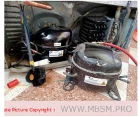
Mbsm.pro, Compresor, tca35712801, fc150nama, refrigerator, lg, 1/5 hp, r600
