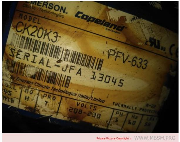
Compressor, Copeland, Ck20k3pfv, 20000 btu, 5040 kcal, 5861 w, 9.6 AC Compressor, Copeland, Ck20k3pfv, 1.5 hp
