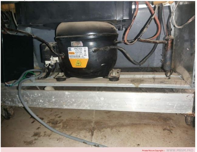
Mbsm.pro, Compressor, hpk190A, 1/4 hp++, 1/3 hp-,R600,HMBP, 220/240V, 50Hz, 12.11 cc , unionaire, UR-350, 340 L, R600a/48q, 0.87 A
