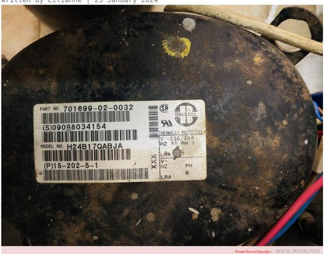
Mbsm.pro, Bristol, Compressor, H24B17QABJA, 17000 btu, 1.5 hp, r22, Capillary Size (0.060), Capillary Length 33″
