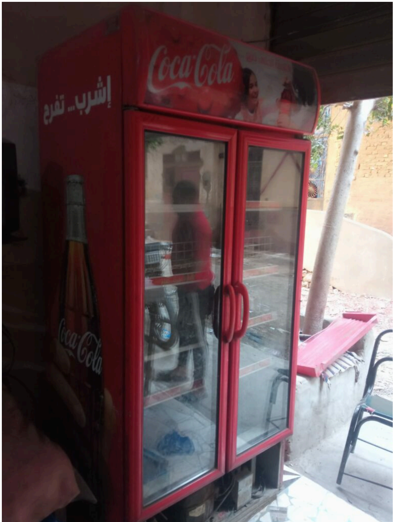
Mbsm.pro, CRC-1000SWL, CRC1000SWF02-C12-06790, COCA COLA, 2-DOOR, 1000L ,COMMERCIAL, GLASS, DISPLAY, FRIDGE, R-404a, 700 g, Compressor, SC15D, 1 hp, hbp
