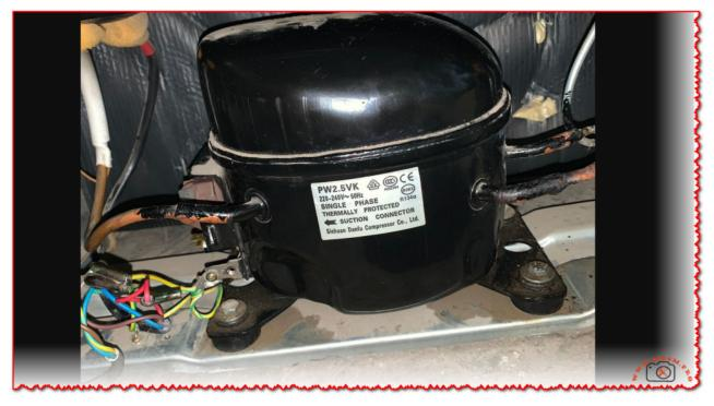
Mbsm.pro, Pw2.5vk, 1/12 hp, Refrigeration, Compressor, R134a, 220~240v Ac 50hz, Mbp/lbp, Sichuan Danfu Compressor
