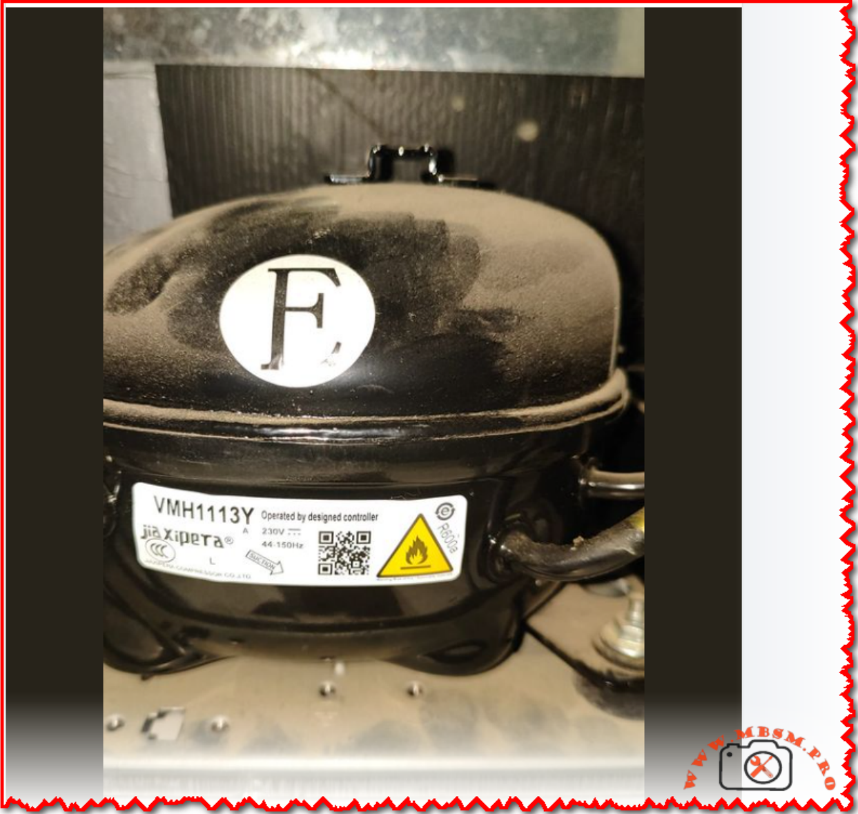
Mbsm.pro, Inverter, BLCD, compressor, refrigerator, R600a, JIAXIPERA, VMH1113Y, 1/6 hp, r600a, lbp
