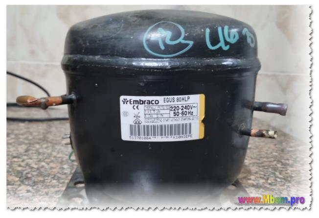
**Embraco EGUS 80HLP** compressor along with its specifications and details related to **LBP (Low Back Pressure)** applications:
