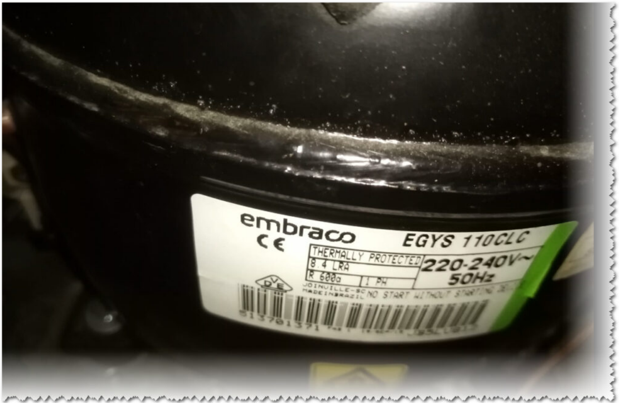
Mbsm.pro, Compressor, Embraco, EGYS110CLC, 1/3 hp, 1bp, r600a, 263 w, 1.1a
