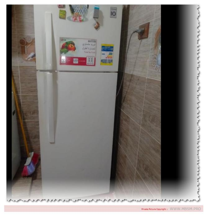
Mbsm.pro, REFRIGERATOR-FREEZER, GR-B392RQCC, 364L, compressor, 1/5 hp, r134a(125g), 1.4 A, 1p/220v
