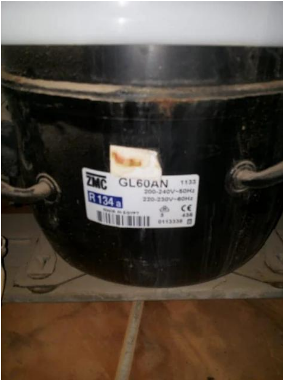
Compressor, ACC, Cubigel, GL60AN, R134a, 220-240V, HMBP, 1/6HP
