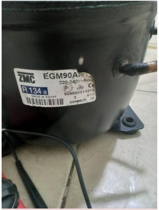
Private Picture Copyright: WWW.MBSM.PRO ZMC EGM90AZ compressor, which is a 1/4+ HP, R-134A, low back pressure (LBP) compressor designed for household applications Here are the details:**Manufacturer**: ZMC (Zanussi Misr Compressor Manufacturing Co. S.A.E) **Model**: EGM90AZ Refrigerant: R134a Application: LBP (Low Back Pressure) Evaporating Temperature Range: -30°C to -10°C Horsepower: 1/4Hp Weight: 150g. Freezer Capacity: 260L Cross, 235L Storage Voltage: 220V-50Hz Current: 1.2A
