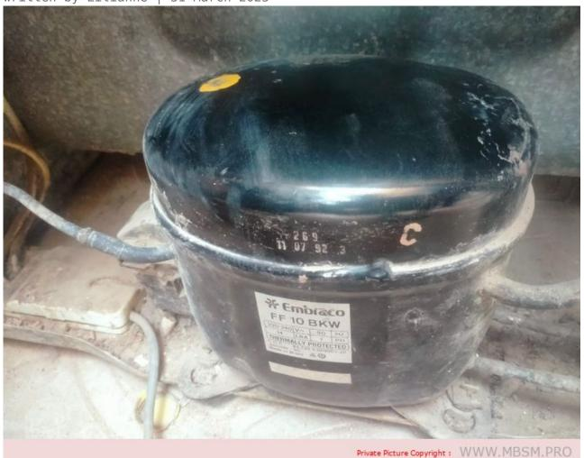
FF10BKW appears to be a compressor model manufactured by Embraco . It is a 1/4+
