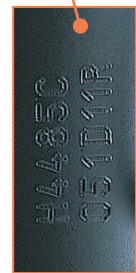
Fig.1 Needle print coding on compressor housing and country of origin on type label
