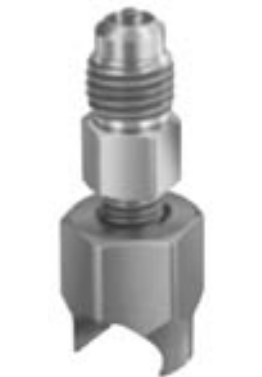
Steel pin with core, penetrates line and is locked into valve body in one operation, simply by tightening cap.
