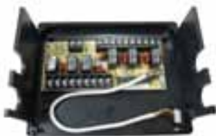
RE392 ZONE RELAY BOARD WITH LOW VOLT CABLE
