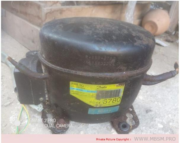
103G6780, compressor Secop / Danfoss FR8.5G, LBP / HBP - R134, 220 - 240V / 1 / 50 Hz, discharge 7.95 cm3, motor type RSIR/CSIR, oil type POE, oil charge 450 cm3, 126 W at -25 / 55° C, LRA 8.2 A, maximum refrigerant charge 900 g, height: 196 mm, weight 10.6 kg
