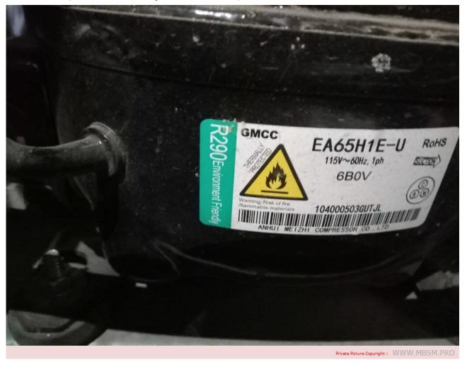
Mbsm.pro, Compressor, EA65H1E-U, 1/3 hp++, mbp, r290, freezer, with two doors, GMCC Refrigeration Compressor
