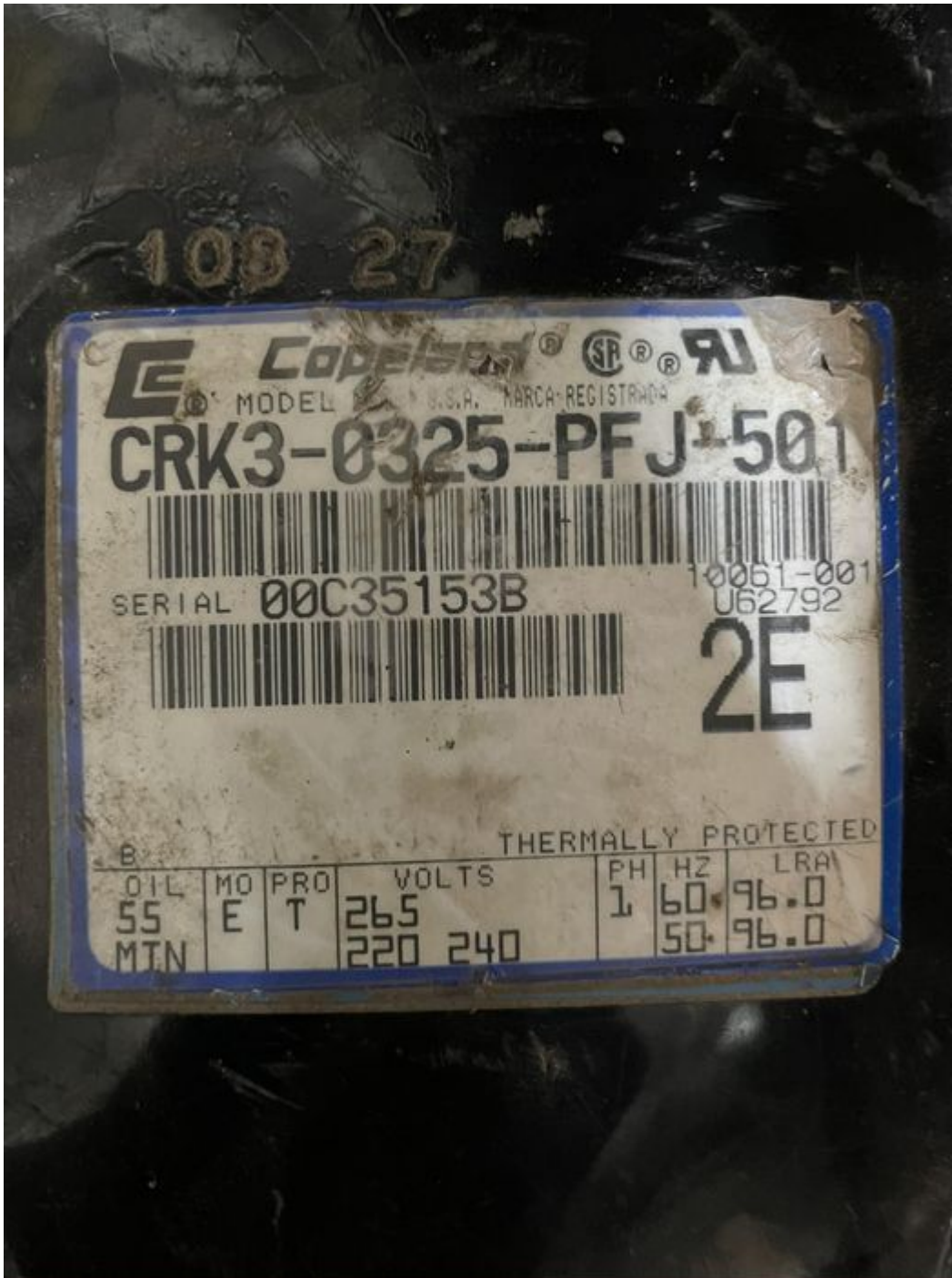
Compresor, Copeland, Hermetico, CRK3-0325-PFJ, 3.5 T, HCFC, R22, 50 Hz, 1 PH, 220/240 V, 3.25 hp, 40.600 BTU
