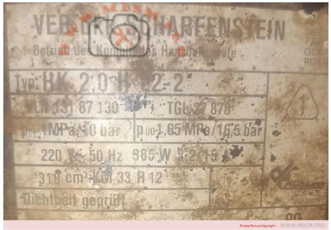
Mbsm.pro, Compressor, tgl27878, tgl27 878, VEB dkk Scharfenstein,1993, R12, 3/8 hp++, 1/2 hp-, 385 w, Cooling Compressor, 0 °C 10 °C, Replaced by GP12TB
