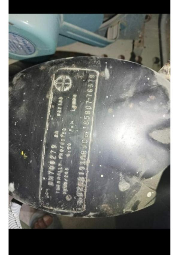
Mbsm.pro, Bristol, Compressor, H20B243ABC, 24000 btu, r22, 220 v 50hz, 2 ton, D6789205, AB5522G,
