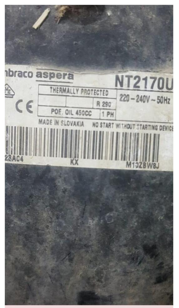
Mbsm.pro, Embraco, Aspera, NT2170U, compressor, LBP, R290,, 220 - 240V/1/50Hz, 1- HP,
