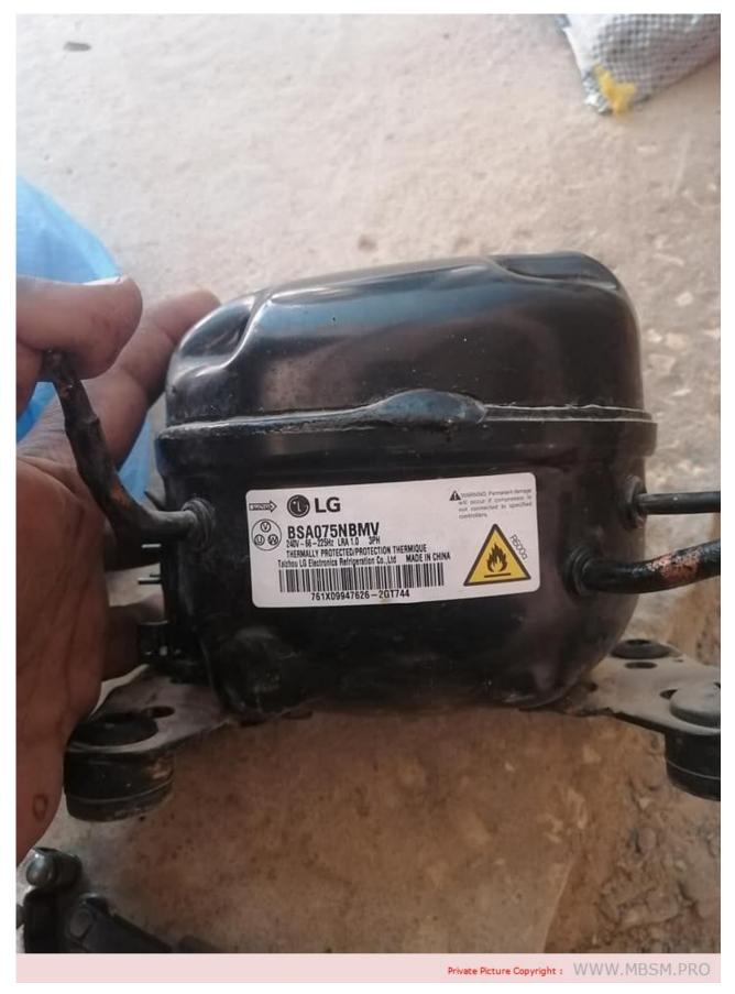
Mbsm.pro, Compressor, Lg, bsa057nbmv, BLCD, Inverter, serie BS, 540 L, ENIEM, TN2000, Nofrost, r600a, 1/5 hp
