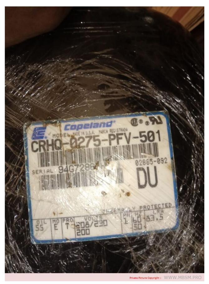
Mbsm.pro, Hermetic, Copeland, Compressors, CRHQ-0275-PFV, crhq0275pfv, crhq-0275-pfv-501, crhq0275-pfv-501, crhq0275-pfv, 4 Hp, r22, 33800 btu
