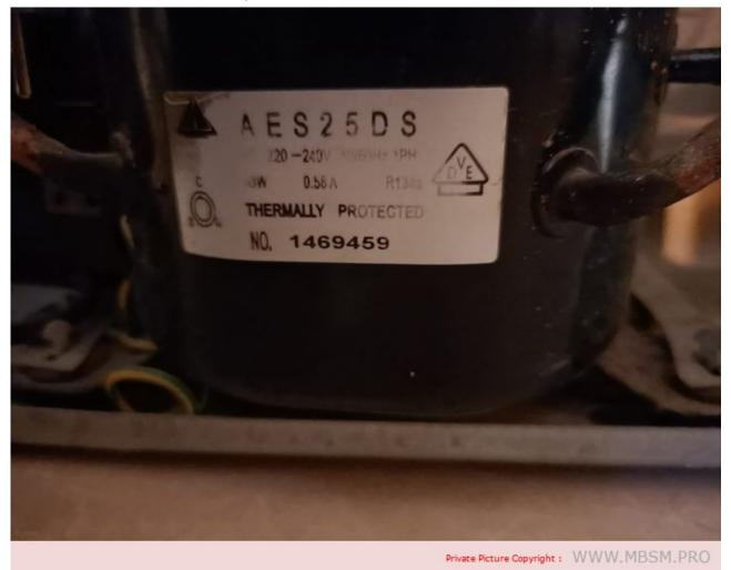
Mbsm.pro, small office, refrigerator, compressor, aes25ds, 1/10 hp, r134a
