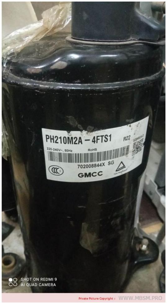
The PH210M2A-4FTS1 is a rotary compressor manufactured by GMCC. It is a hermetic
