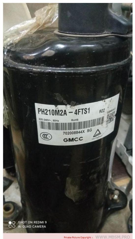
The PH210M2A-4FTS1 is a rotary compressor manufactured by GMCC. It is a hermetic
