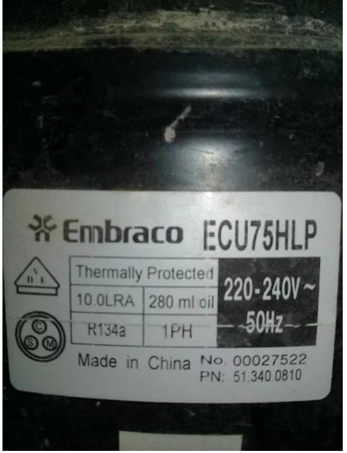
RT 1320 windsor, windsor refrigerator, 13.2 Feet/cub, 400 L, Compressor, Embraco, ecu75hlp, 250 w, 1/4 hp, Lbp, r134, 180 g, 7.5 cm<sup>3</sup>, 220-240 V at 50 Hz
