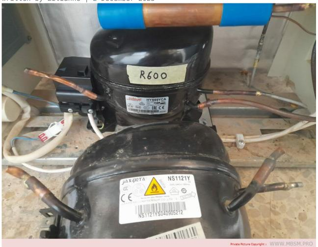
Mbsm.pro, Replaced, Jiaxipera, NS1121Y, 1/4 hp++, 1/3 hp-, 214Kcal, R600a, 220V, with, Compressor, hys69yq, 1/4 hp, lbp, r134a, HiTech, refrigerator, HSA 47542/1, SN-T, C467 — HC, Beko, 451 L, R600a, 64G
