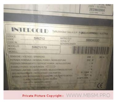
Mbsm.pro, SWZ12, 000DK02D, 2eDM02000, Intercold, Freezer, swz1/170, 222 w, 230v, Compressor, 1/4 hp, R134a, 210 G, 290 L, Intercold horizontal freezers for frozen
