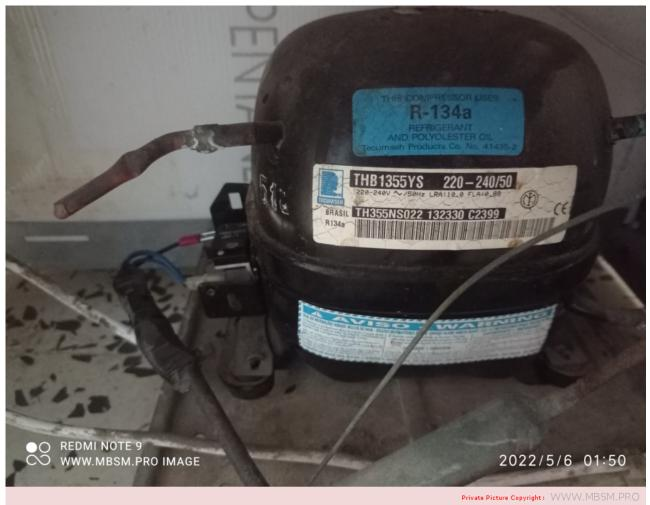
Mbsm.pro, Freeser, Ariston, ECH240s1, 240 L, Compressor, TECUMSEH BRASIL, THb1355y, 1/5 hp, LBP, R134A, 100g, replaced by, egm70af, gl70aa, capillarie 0.026, 1.2 m, Alert -10 Mbsm.pro, Air Conditioner, GAC-C12A4, General Gold, 12000 btu/h, Cooling, Heating, 1.5 hp, 1 ton, R22, 580 g, T1
