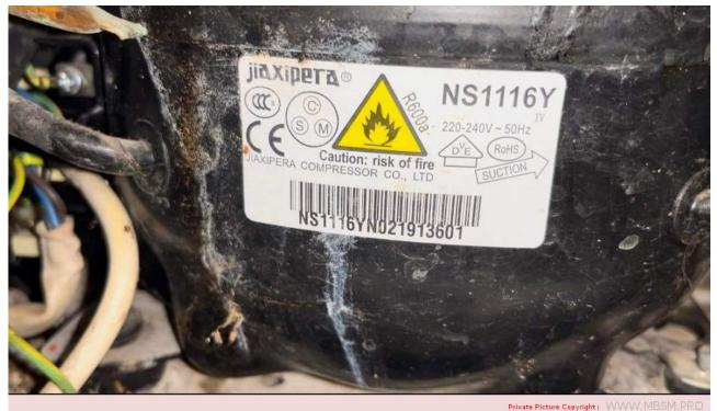
Mbsm.pro, Compressor, ns11116,1/5 hp, Lbp, R600A, 186 W, 220-240~/50hz, R600, 10.50cc, JIAXIPERA Compressor
