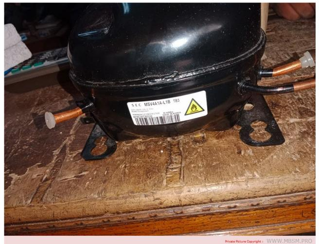
Mbsm.pro, compressor, MSV4A1A-L1B, inverter, Bldc, 1/5 hp, Samsung , 168 w
