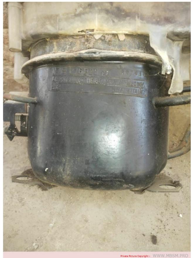
Mbsm.pro, compressor, IRE, L16b22, IREL16b22, 1/5 hp, r12, 180 w, 220v 50hz, Remplacement with 1/4 hp, r134a, Italien compressor
