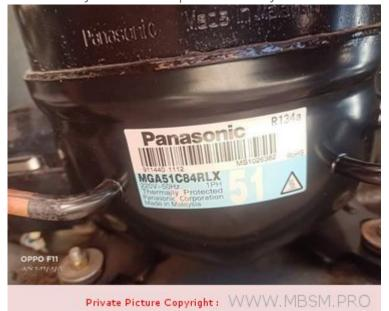
Mbsm.pro, Compressor, MGA51C84rLX, MGA51C68RPU, Panasonic compressor, M Series, Reciprocating Fixed Speed, 180 W, 1/5 Hp, RSCR, 220 V , r134a
