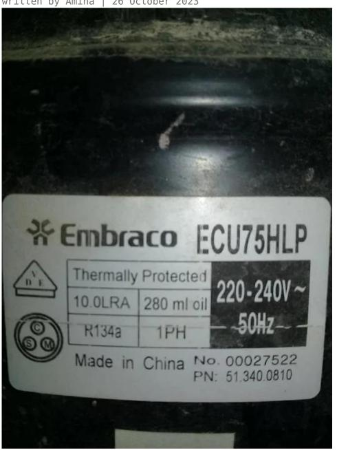
RT 1320 windsor, windsor refrigerator, 13.2 Feet/cub, 400 L, Compressor, Embraco, ecu75hlp, 250 w, 1/4 hp, Lbp, r134, 180 g, 7.5 cm<sup>3</sup>, 220-240 V at 50 Hz
