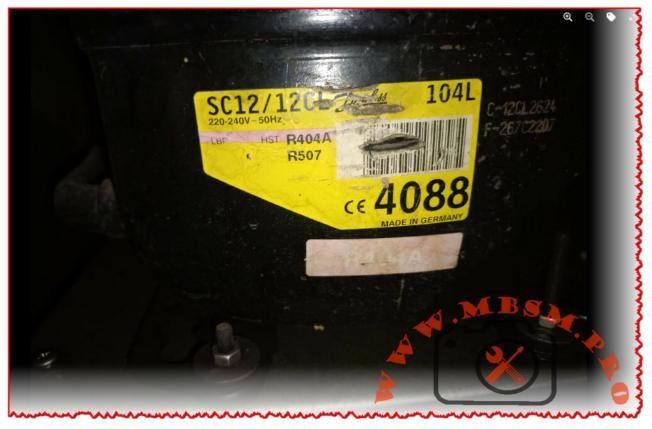
Mbsm.pro, Compressor, SC12/12CL, 104l 4088, Compressor twin, SECOP, 104L4088, R404A/R507, 3/8 hp, mhbp
