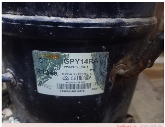
Mbsm.pro, Cubigel, Compressor, GPY14R, R134a, HMBP, 3/8 HP, HMBP, 14.32cc, High Efficiency,
