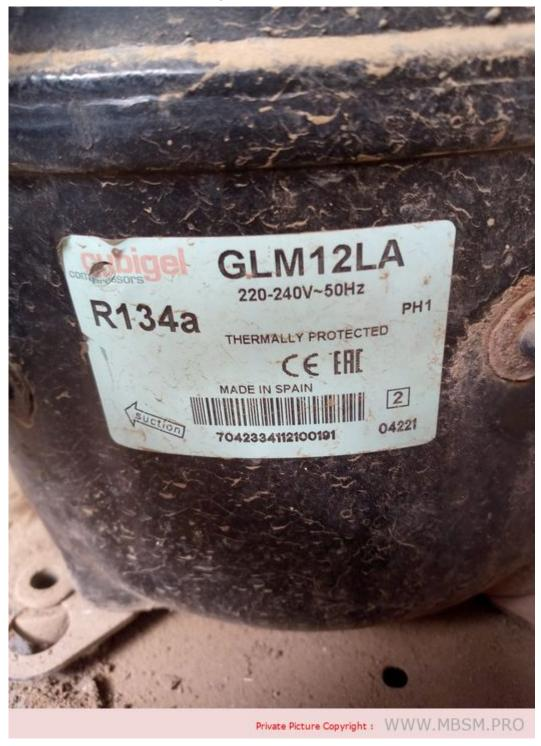
Mbsm.pro, Compressor, Cubigel/ACC, GLM12LA, R134A, 3/8 Hp, Lbp
