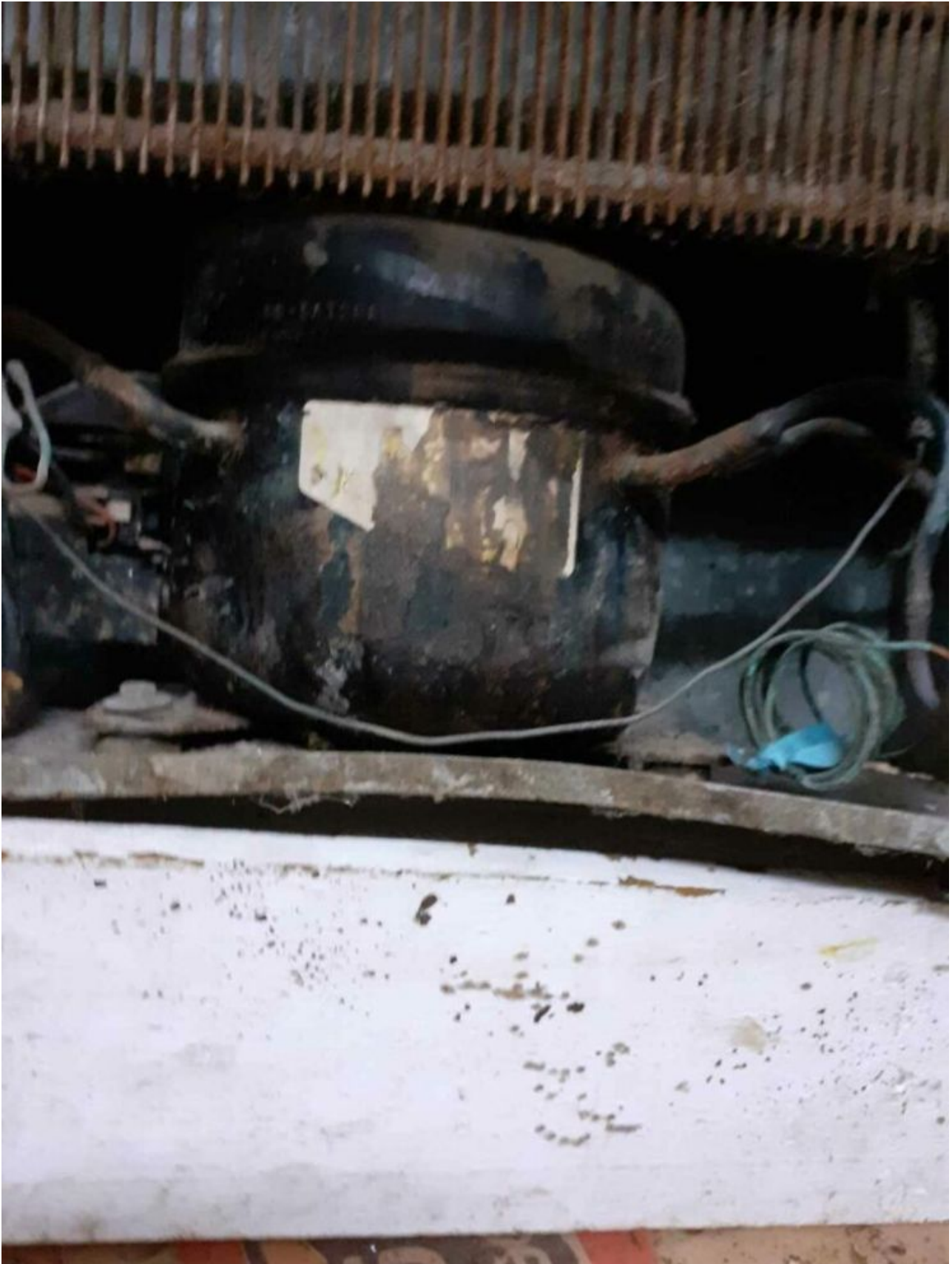
Mbsm.pro, Compressor, FR7.5G, R-134a/r12, 1/5HP, 50/60Hz, Danfoss
