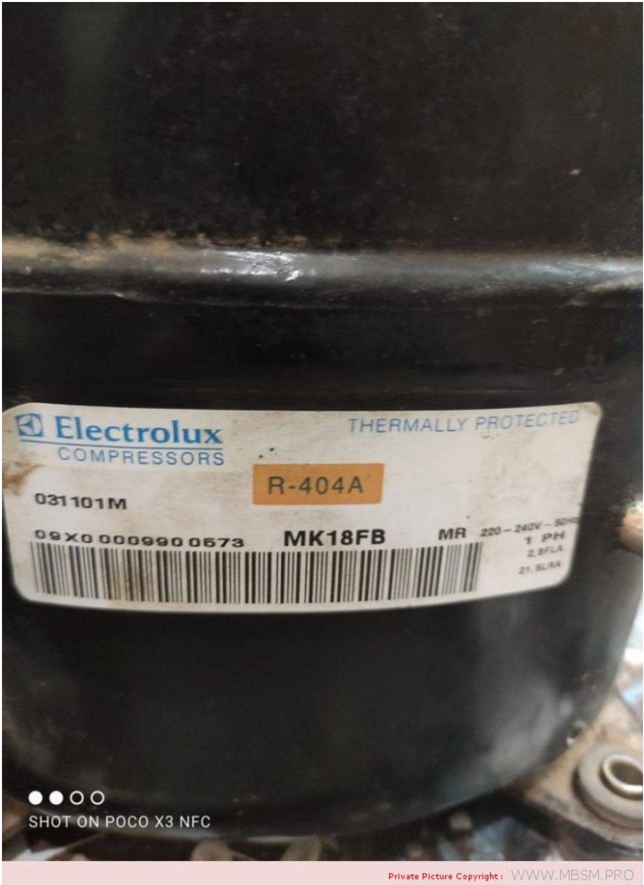
Electrolux Professional Compressor, R404a/R507, MX18FB, 220-240V, 50Hz, 17,3kg, 5/8HP, 571W, MX18 FB, CUBIGEL, LBP, HERMETIC COMPRESSOR, Zanussi ALF1103 Fridge
