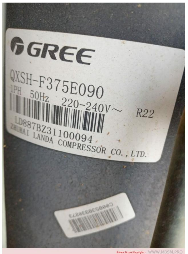
Mbsm.pro, compressor, Gree, Air conditioner, OXSH-F375E090, OXSH-F375, 22100 btu, 37.50 cm3, 6477 w, capasitor 60 uf, 1.8 ton, 2.8 hp, 220 v, 1ph
