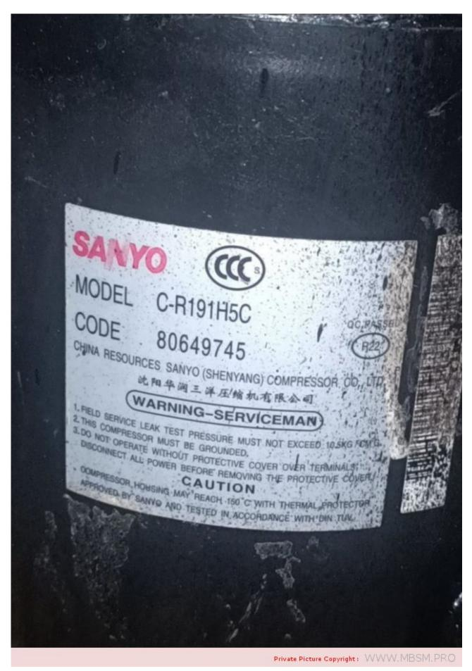
Mbsm.pro, Compressor, C-R191H5C, Sanyo, 24000BTU, air conditioner compressor, r22, 2 ton
