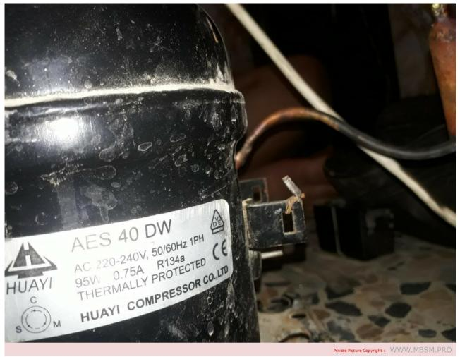
Mbsm.pro, Compressor, AES40DW, COMPRESSOR HUAYI, 1/8 HP, R-134, 95 w, AES 40 DW, 0.75 A, #AES40DW
