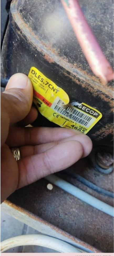
Mbsm.pro, compressor, dle5.7cnt , Secop, Danfoss, 102H4685, 1/4 hp++, 1/3 hp-, r290
