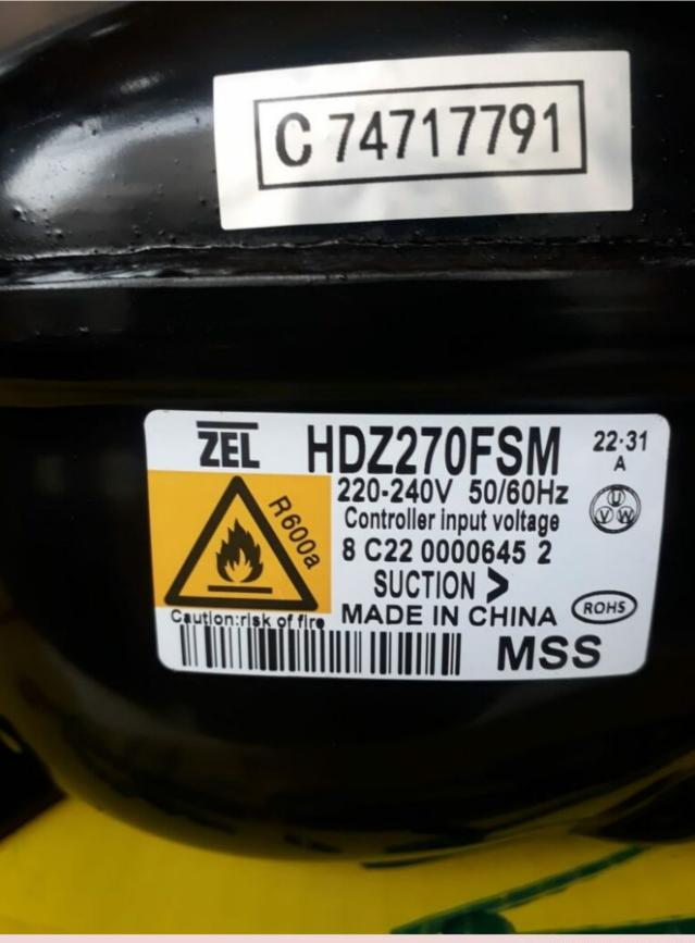
Mbsm.pro, Compressor, hdz270fsm, Inverter, Bldc, Variable speed, form 80 w to 250 w, 1/3 hp, Carte Controller devise
