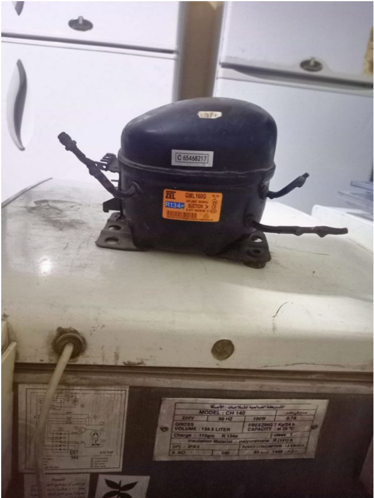
Mbsm.pro, Compressor, ZEL, GML160G, 1/6 hp, 129 w, LBP, R134a, 220-240V, KONOR CATALOG
