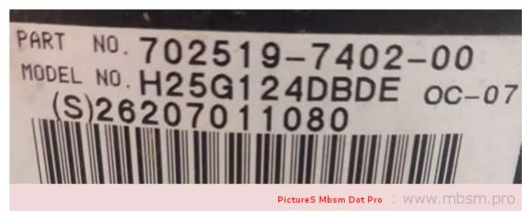
www.mbsm.pro, cOMPRESsOR A/A ,124MBTU, 220V/380v, 3HP, H25G124DBDE, BRISTOL
