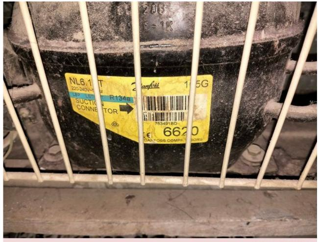
Private Picture Copyright : WWW.MBSM.PRO Mbsm.pro, Compressor, NL6.1FT, SECOP, 105G6620, DANFOSS, 1/6 hp, Lbp
