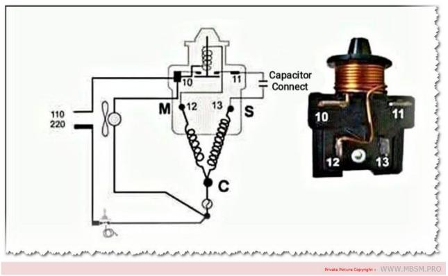
Mbsm.pro, Danfoss, compressor, relay, connection, Refrigeration
