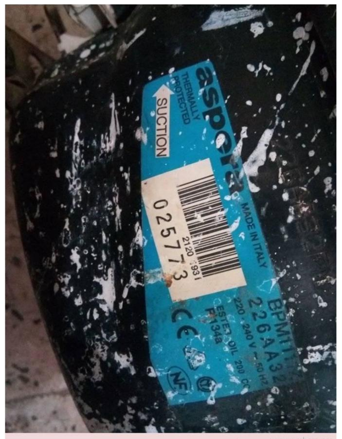
PictureS Mbsm Dot Pro : WWW.mbsm.pro Compressor Bpm111z , r134a 1/6hp ,5.6cc, 240v 50hz ,ASPERA, EMBRACO
